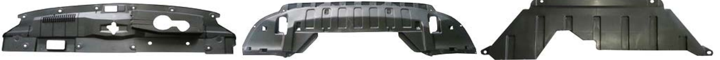
1 ENGINE COVER UPPER (WATER TANK COVER) 2 ENGINE COVER UNDER (FRONT) 3 ENGINE COVER UNDER (REAR)
